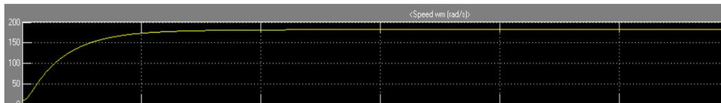
Fig8(b). Speed of DC motor with Fuzzy logic controller
