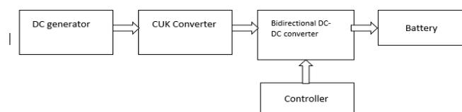
Fig2. Block diagram of BFEV during regenerative braking mode
