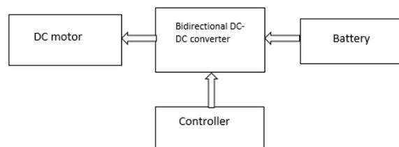
Fig1. Block diagram of BFEV during acceleration mode
