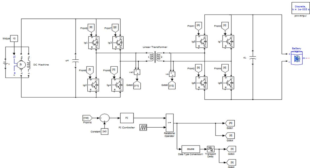
**Fig4.** Simulink model of BFEV with PI controller during acceleration mode
